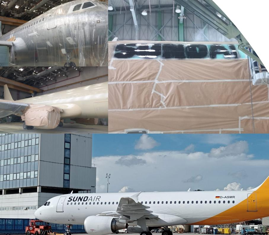
A modern and state-of-the-art painting bay, allows Atitech to satisfy all the customer needs in terms of sanding, stripping and painting, in compliance with the most stringent environmental regulations.
